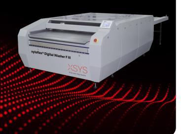
Mid web format, suitable for processing high quality digital and conventional photopolymer plates up to a maximum size of  $1020 \text{ mm} \times 1200 \text{ mm} (40.2^{\circ} \times 47.0^{\circ})$
